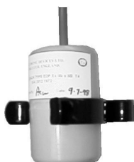
EDP GAS SENSOR
